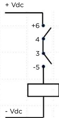
The load is disconnected when the relay is de-energized
